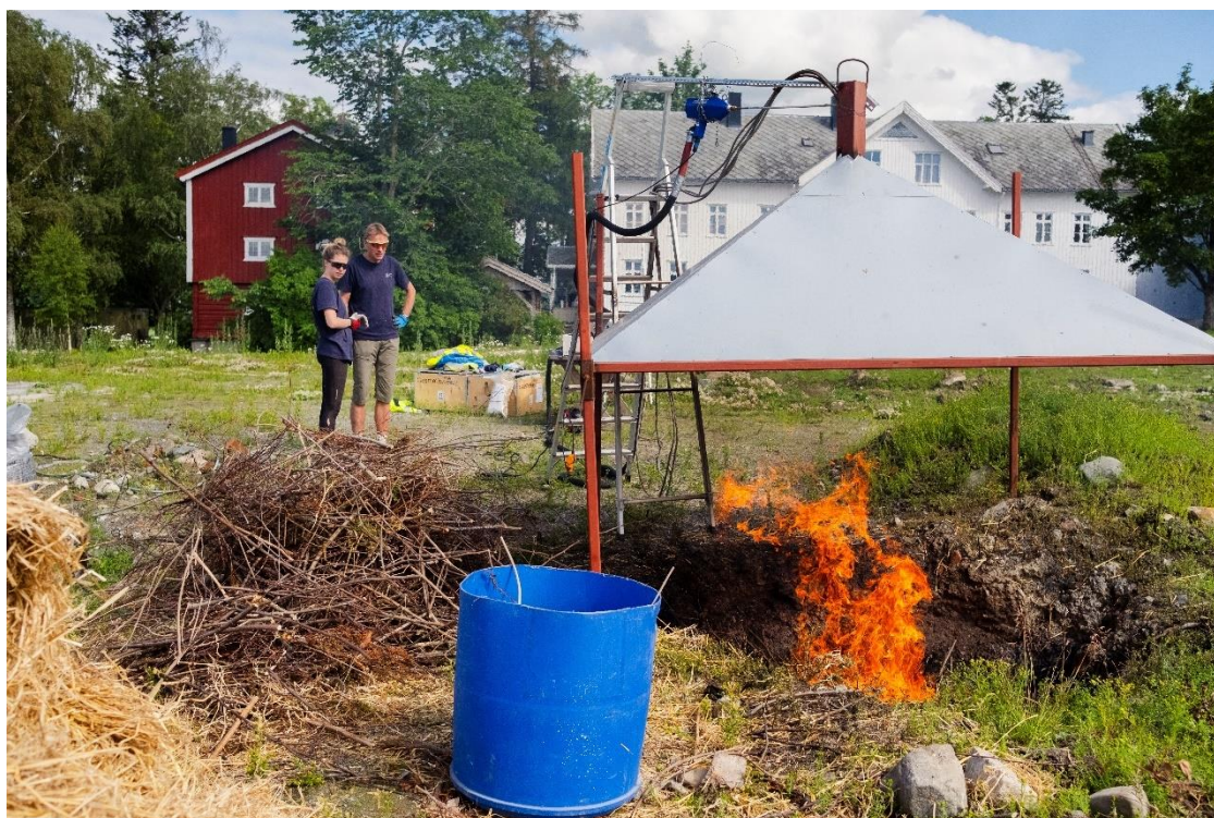
Figure 2 Kiln at Mære Landbruksskole with roof to collect gases.
